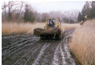
The Marshwalker is a small backhoe with extra wide rubber tracks designed to put less pressure on the Marsh.
